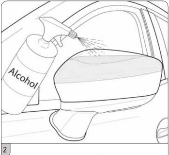
Fold down the top lip of film and spray alcohol then fasten down with squeegee.
