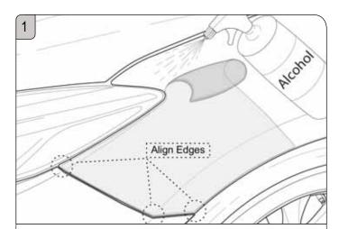
Prep surface for film placement. Spray baby shampoo mix and position film on fender, align edges properly
